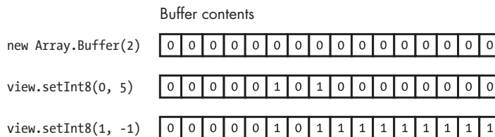
Figure 10-1: The array buffer after two method calls
