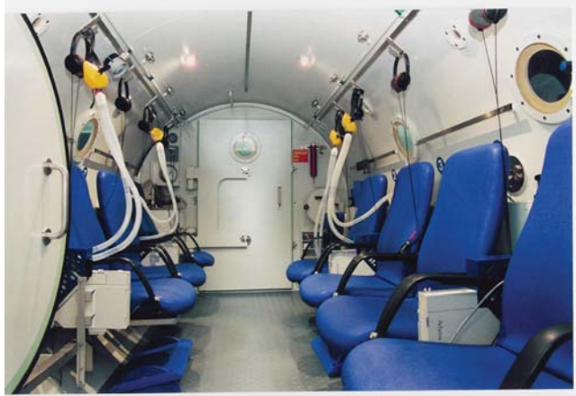
Figure 22.2 Multiplace chamber using compressed air and 100% oxygen hood. (See color plate section for the color representation of this figure.)
