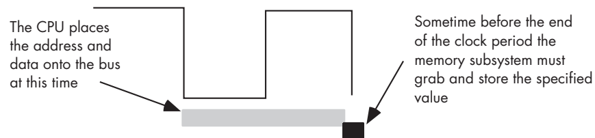
Figure 6-18: A typical memory write cycle
