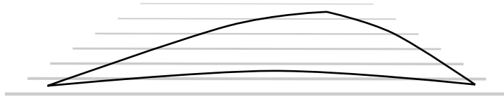
Figure 5-10: Bending the normals gives the triangle a bent shape so far as the lighting calculations are concerned.
