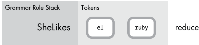
Figure 1-19: The parser matches the SheLikes rule and reduces.
