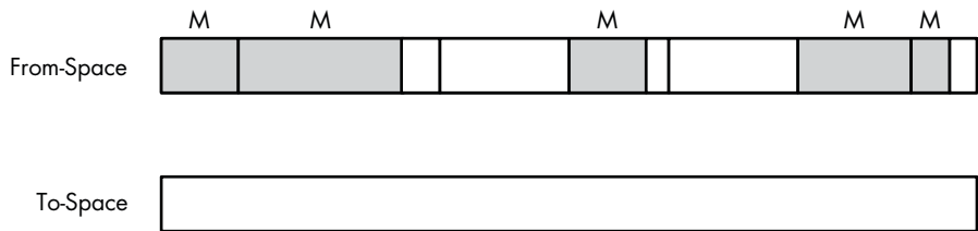
Figure 12-10: The semi-space algorithm uses two heaps, one initially empty.
