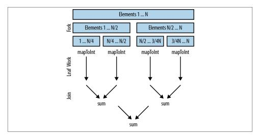
Figure 6-2. Decomposing and merging using fork/join
