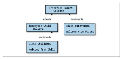
Figure 4-4. A diagram showing the inheritance hierarchy at this point
