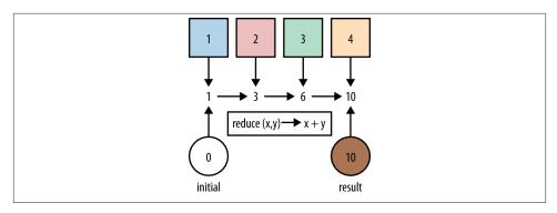
Figure 3-8. Implementing addition using the reduce operation
