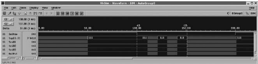
Fig. 14.10 Simulation of a delay line using enabled rtran resistor models
