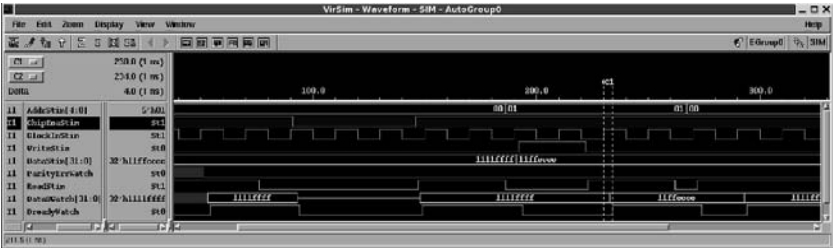
Fig. 5.5 Cursory simulation of single-port Mem1kx32 with separate read and write ports
