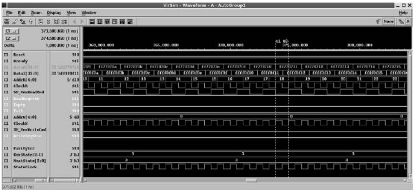
Fig. 20.14 Zoomed-in view of synthesized FIFO netlist simulation, showing individual 32-bit word transfers
