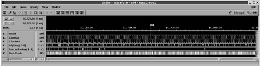
Fig. 18.9 The source PLL 1 × verilog model: Lock-in detail near end of 20 us simulation
