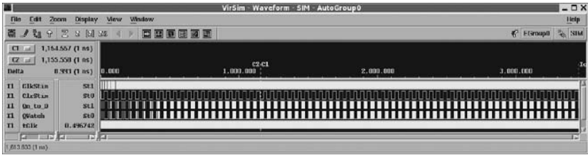
Fig. 17.6 Overview of the DFFC simulation with slowly increasing clock frequency
