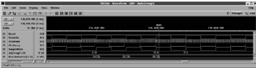
Fig. 20.12 Zoomed-in view of synthesized PLL netlist simulation, showing individual serial clock cycles
