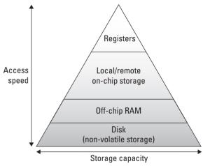
**Figure 6.7.** FPGA compute core's memory hierarchy with local/remote storage in place of cache.
