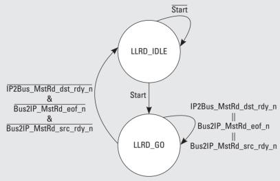
Figure 6.17. Bus master read request finite state machine.
