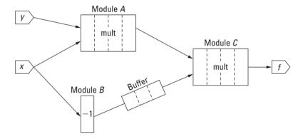
**Figure 6.3.** High-throughput network to compute xy(x-1).
