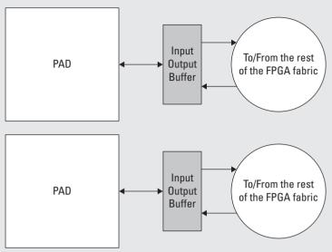
Figure 2.21. Xilinx Select Input/Output buffer (IOB) tile for connections between FPGA fabric and the pad on the FPGA device.
