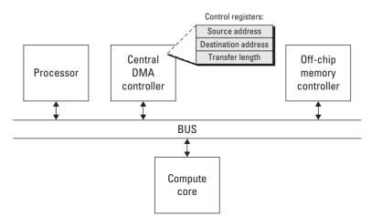
Figure 6.12. Central DMA controller to offload memory transactions from the processor.
