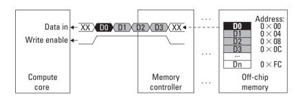
**Figure 6.13.** Burst transfer of four 32-bit sequential data words from off-chip memory to a compute core.
