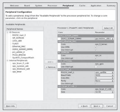
Figure 3.21. Peripherals needed for the "hello world" Linux system on the Xilinx ML510 development board.
