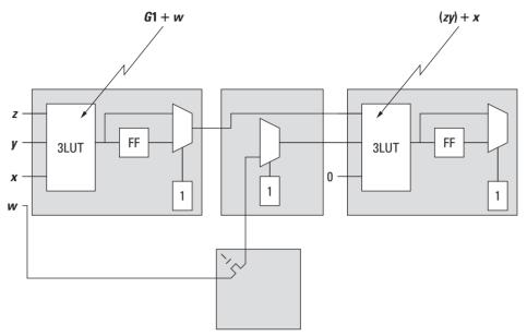
**Figure 2.16.** Illustration of f(w, x, y, z) placed and routed.
