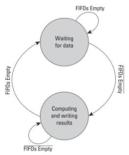
**Figure 6.5.** Wait/compute states of Kahn process network finite state machine.
