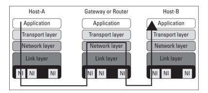
**Figure 7.2.** Two hosts communicating with TCP/IP.
