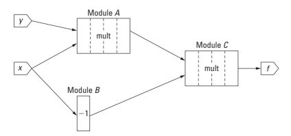
**Figure 6.1.** A simple network used to compute xy(x-1).
