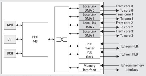
**Figure 2.23.** PowerPC 440 processor block diagram showing the available interfaces between processor and FPGA fabric.
