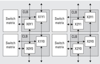
Figure 2.20. Virtex 5 CLB block diagram of the interconnection between each slice in the CLBs and their connection to the switch matrix.
