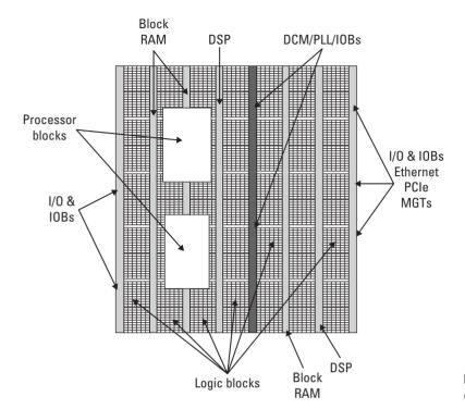
**Figure 2.11.** A high-level view of a Platform FPGA.
