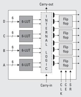
Figure 2.19. A block diagram of a Virtex 5 logic slice with four 6-LUTs and four flip-flop/latch storage elements.
