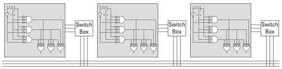
Figure 2.8. Simple CPLD device organization example.
