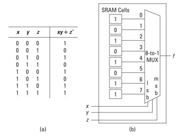
Figure 2.9. Three-input function generator in (a) truth table and (b) look-up table form.
