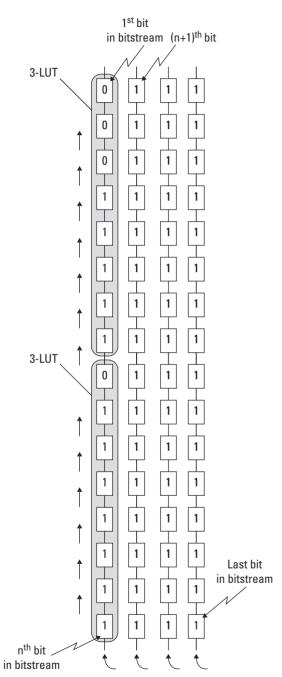
**Figure 2.17.** Illustration of f(w, x, y, z) placed and routed.
