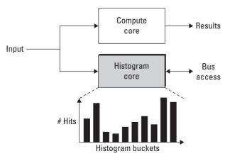
Figure 6.14. Streaming I/O compute core plus parallel data acquisition (histogram) core.
