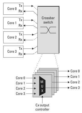
**Figure 6.15.** A four-port crossbar switch and its internal representation based on multiplexers.
