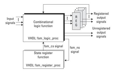
Figure 2.12. The VHDL process with the corresponding sequential digital circuit for finite state machines.
