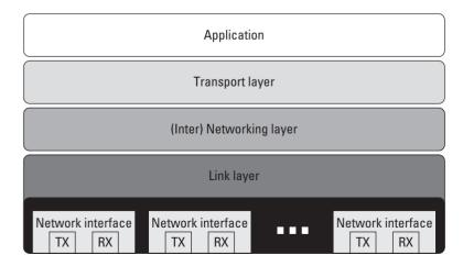
**Figure 7.1.** A network protocol stack.
