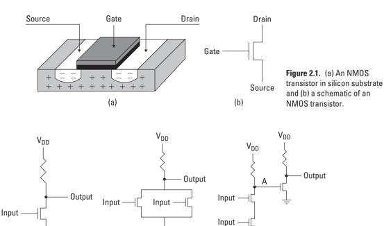
Figure 2.2. An NMOS (a) NAND gate, (b) NOR gate, and (c) AND gate.
