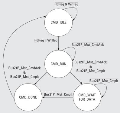
Figure 6.16. Bus master control finite state machine.
