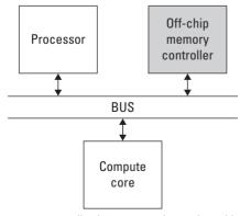
**Figure 6.10.** The memory controller is connected to a shared bus to support requests by any core on the bus.
