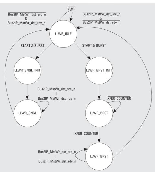
Figure 6.18. Bus master write request finite state machine.
