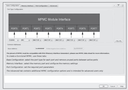
Figure 6.22. Xilinx Multi-Port Memory Controller configured with two ports: PLB and NPI.
