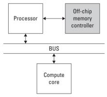
Figure 6.9. The processor is connected directly to the memory controller.
