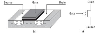
Figure 2.4. (a) A PMOS transistor in silicon substrate and (b) a schematic of a PMOS transistor.
