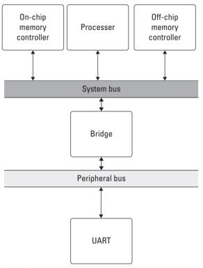
**Figure 3.9.** Block diagram of the base system consisting of a processor, on-chip and off-chip memory, and a UART.
