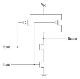
Figure 2.5. A simple CMOS NAND circuit.
