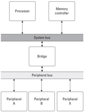
Figure 3.8. The two bus process-memory model used to support parallel, independent high-speed and low-speed communication.
