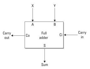
Figure 3.1. Implicit module description of a full adder.
