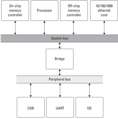
**Figure 3.10.** Block diagram of the base system with the additional cores: networking, USB, and I2C.
