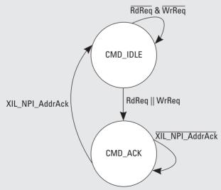
Figure 6.19. Native Port Interface control finite state machine.
