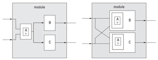
Figure 3.4. (a) Original design and (b) modified design with lower coupling.
