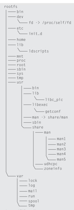
Figure 3.16. Typical bare-bones layout of FHS root filesystem.
