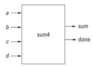
Figure 3.12. The top-level component to add four numbers.
