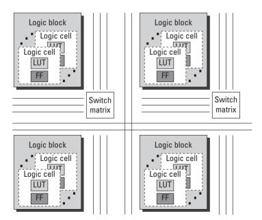
Figure 2.10. A high-level block diagram of a simple FPGA consisting of logic blocks, logic cells, storage elements, function generators, and routing logic.
