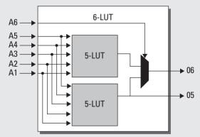
Figure 2.18. The Virtex 5 6-input LUT actually is built from two 5-input LUTs with the sixth input controlling a mux between the two LUTs.
