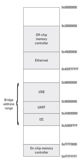
**Figure 3.11.** One possible address map for the theoretical two-bus system with networking, USB, I2C, and UART.
