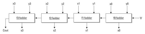
Figure 3.3. Four formally defined modules to generate a 4-bit full adder from 1-bit full adders.
