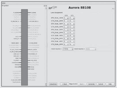
Figure 7.4. Lane to transceiver mapping.
