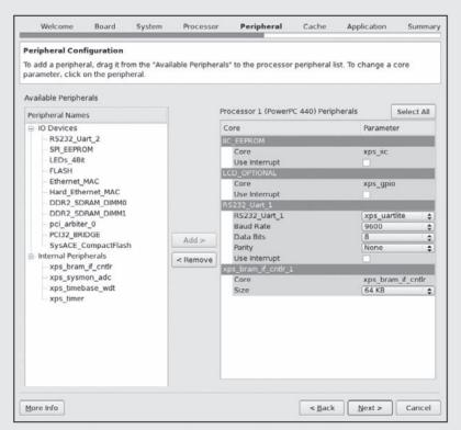
Figure 7.5. Peripherals needed for the I2C EEPROM example on the Xilinx ML510 development board.
