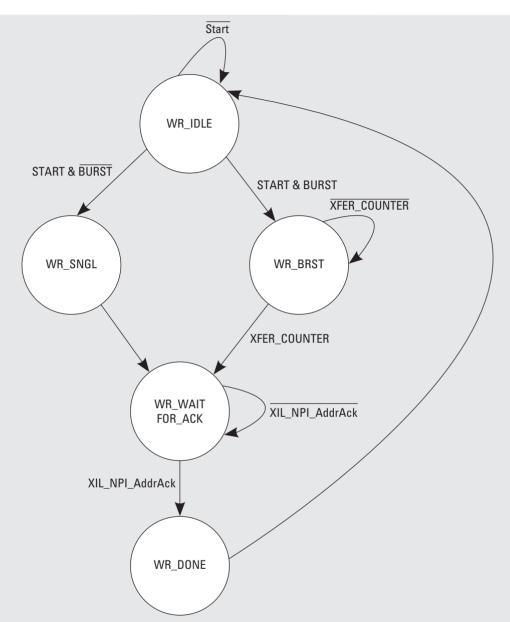
Figure 6.21. Native Port Interface write request finite state machine.
