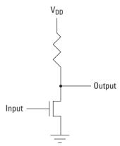
Figure 2.3. Schematic symbol of an NMOS inverter.
