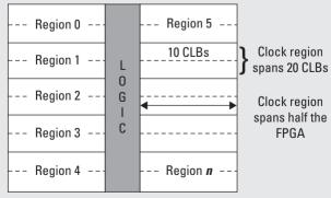
Figure 2.22. Clock regions on an FPGA span 20 CLBs vertically and half of the FPGA horizontally; the number of clock regions varies by chip.
