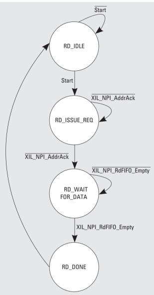
Figure 6.20. Native Port Interface read request finite state machine.
