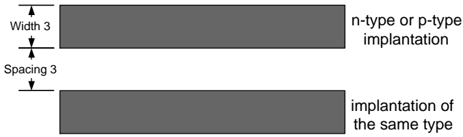
FIGURE 17.6 Design rules for two implantations of the same type.
