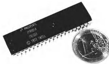
Figure 5.7. The Intel ® I8085, a more modern version of the I8080 ® , had simpler electronics, in particular a single 5 V power supply and an integrated clock generator, a few additional interrupts and a multiplexed address-data bus
