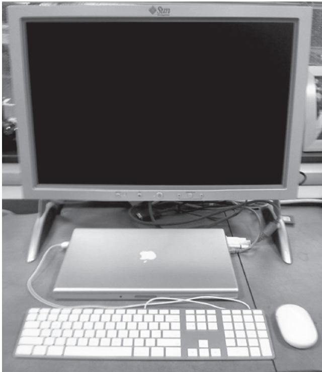
FIGURE 1.5 A desktop computer. The liquid crystal display (LCD) screen is the primary output device, and the keyboard and mouse are the primary input devices. On the right side is an Ethernet cable that connected the laptop to the network and the Web. The laptop contains the processor, memory, and additional I/O devices. This system is a Macbook Pro 15" laptop connected to an external display.
