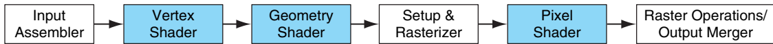
FIGURE A.2.3 Graphics logical pipeline. Programmable graphics shader stages are blue, and fixed-function blocks are white.
