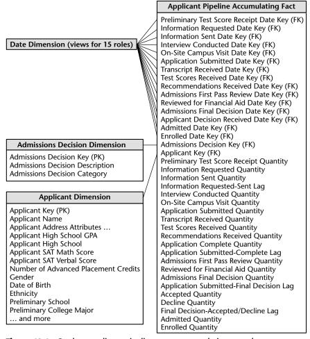
**Figure 12.1** Student applicant pipeline as an accumulating snapshot.
