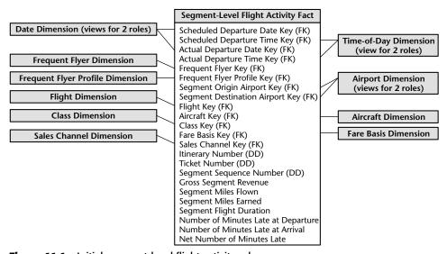
**Figure 11.1** Initial segment-level flight activity schema.
