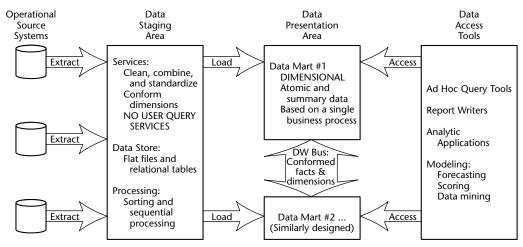
**Figure 1.1** Basic elements of the data warehouse.
