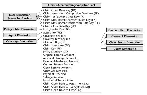
**Figure 15.9** Claims accumulating snapshot schema.
