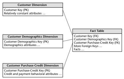
**Figure 6.5** Separate demographic and behavioral minidimensions.
