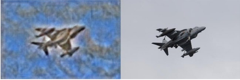
Figure 4-12. Discrimination via a visualization of the HOG description. (Image (c) Carl Vondrick, used by permission.) See also “HOGgles: Visualizing Object Detection Features, Carl Vondrick, Aditya Khosla, Tomasz Malisiewicz, Antonio Torralba, Massachusetts Institute of Technology, Oral presentation at ICCV 2013”
