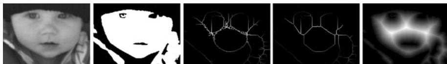
Figure 6-5. Morphological methods to find interest regions. (Left to right) Original image, binary thresholded and segmented image using Chan Vese method, skeleton transform, pruned skeleton transform, and distance transform image. Note that binary thresholding requires quite a bit of work to set parameters correctly for a given application
