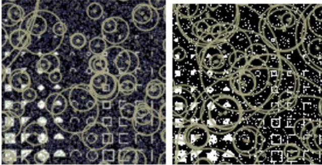
Figure A-9. MSER detector (black on white, white on black, and light gray on dark gray have no detected features)
