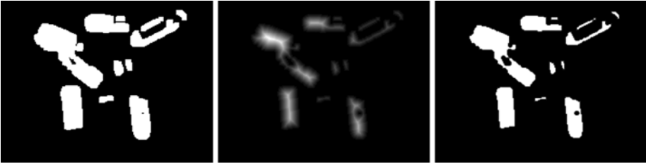
Figure 2-18. Pre-processing sequence: (Left) Image after thresholding and erosion. (Center) EDM showing gray levels corresponding to distance of pixel to black background. (Right) Simple binary thresholded EDM image
