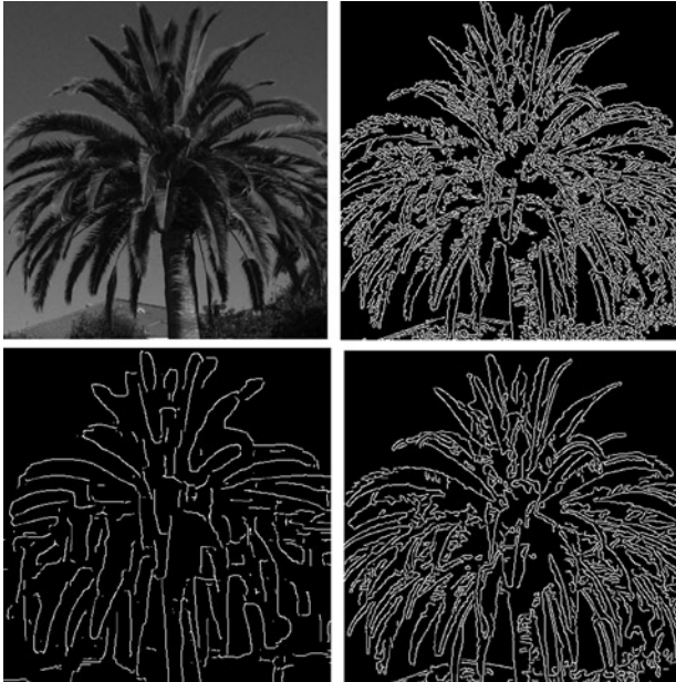
Figure 7-3. (Top left) Image pre-processing for edges shown using Shen-Castan edge detection against ground truth data. (Top right) Over-fitting detection parameters yield too many small edges. (Bottom left) Under fitting parameters yield too few edges. (Bottom right) Relaxed parameters yield reasonable edges
