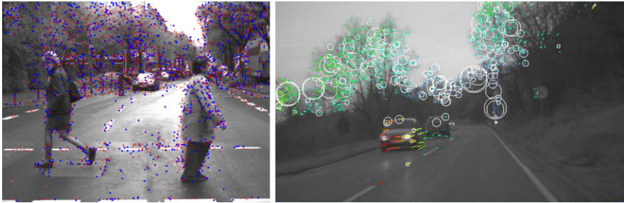
Fig. 9.1 An illustration of DoG scale space keypoints. Left : The detected keypoints in a traffic scene. Right : The keypoints with their disks of influence; the radius of a disk is defined by the scale for which the keypoint has been detected
