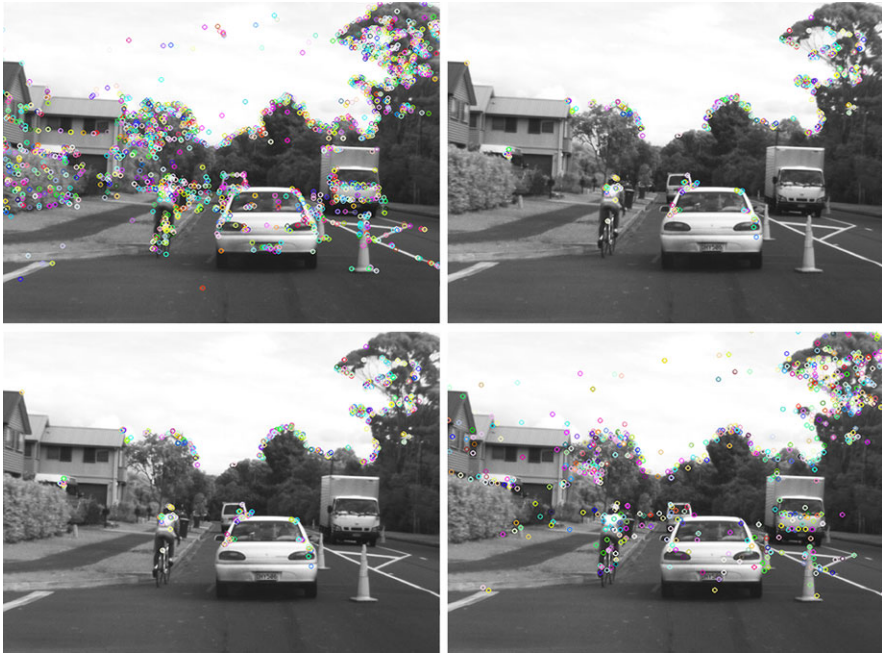
Fig. 9.3 Four keypoint detectors in OpenCV . Upper left : The keypoints detected with FAST. Upper right : The keypoints detected with ORB. Lower left : The keypoints detected with SIFT. Lower right : The keypoints detected with SURF
