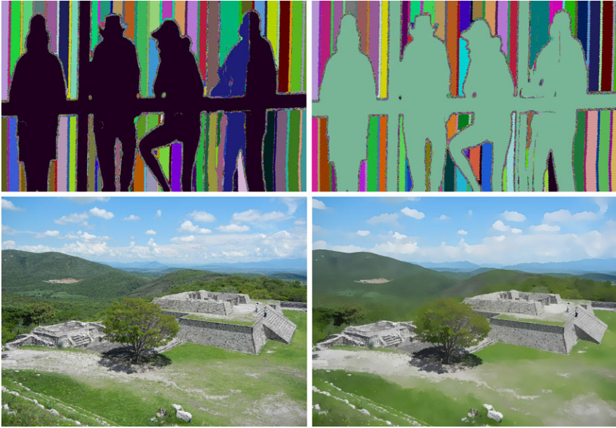
Fig. 5.36 Top : Segmentation results for the image Aussies , where segments are pseudo-coloured rather than shown with the image value identified at the peak. Use of sp = 12 and sr = 19 ( left ), or use of sp = 5 and sr = 24 ( right ). Bottom : The image Xochicalco ( left ) and segmented image ( right ) using sp = 25 and sr = 25
