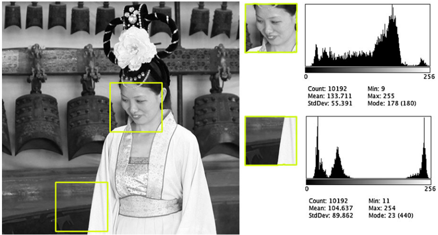
Fig. 1.6 Examples of two 104 \times 98 windows in image Yan, shown with corresponding histograms on the right. Upper window: \mu_{W_1} = 133.7 and \sigma_{W_1} = 55.4 . Lower window: \mu_{W_2} = 104.6 and \sigma_{W_2} = 89.9
