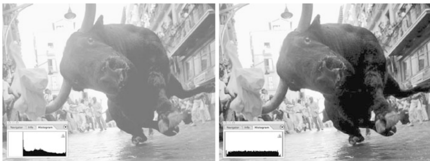
Fig. 2.2 Left: Input image RagingBull (in the public domain) with histogram. Right: The same image after histogram equalization
