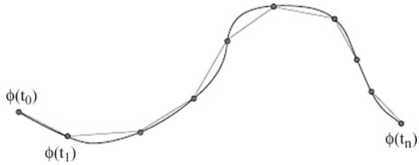
Fig. 3.16 A polygonal approximation of an arc defined by points \phi(t_i) on the arc
