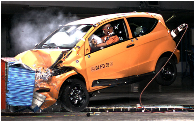
Fig. 6.3 The analysis of a car crash test (here at Daimler A.G., Sindelfingen, Germany) was based (in 2006) on high-resolution images captured at 1,000 pps
