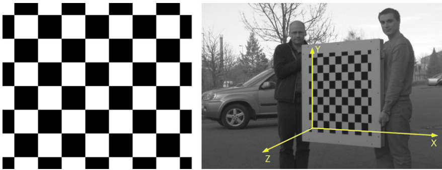
Fig. 6.18 Left: A 2D checkerboard pattern as commonly used for camera calibration. Right: A portable calibration rig; visible light reflections on the pattern would be a drawback when analysing recorded images of a calibration rig. Where is the world coordinate system?
