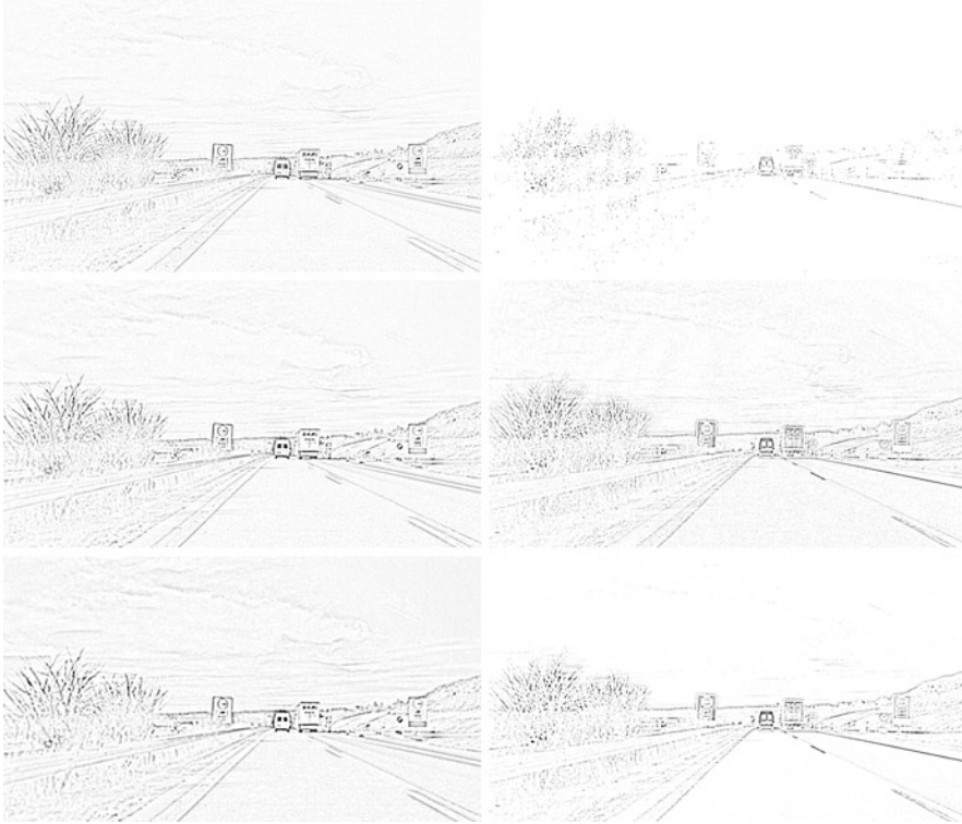
Fig. 2.28 LoG (left) and DoG (right) layers of image Set1Seq1 are generated for \sigma = 0.5 and a_n = 1.6^n for n = 0, \dots, 5 , and the figure shows results for n = 1, n = 3 , and n = 5
