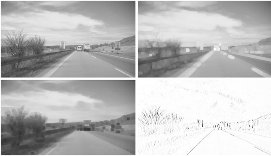
Fig. 2.4 Top, left: Original image Set1Seq1 with N_{cols} = 640 . Top, right: Local maximum for k = 3 . Bottom, left: Local minimum for k = 5 . Bottom, right: Local operator using the 3 \times 3 filter kernel shown in the middle of Fig. 2.5
