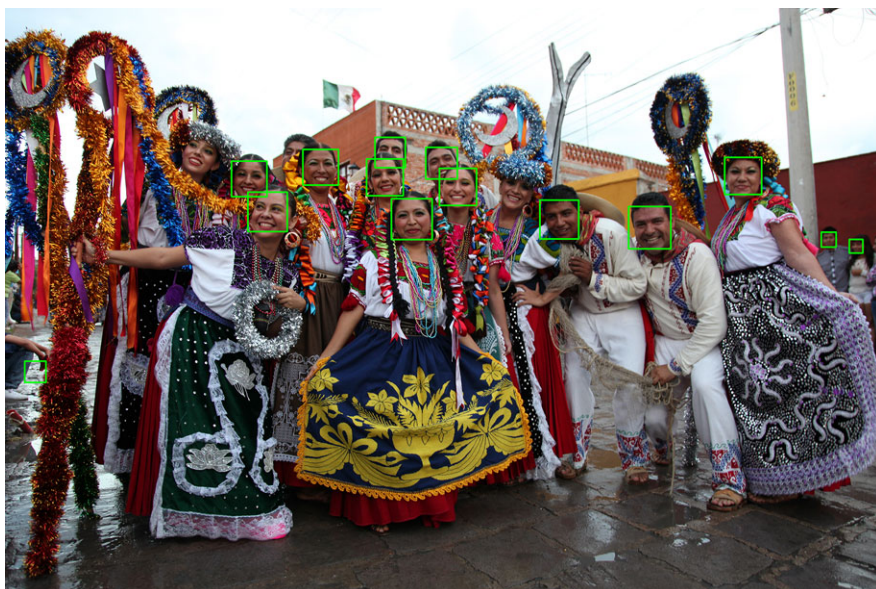
Fig. 10.12 Variation in sizes of faces in the image Michoacan . The applied face detector detects larger faces when using larger masks and smaller faces (see the two on the right ) by using the same masks but with reduced size. There are two false-negatives here; it appears that the used strong classifier is trained for “visible forehead”
