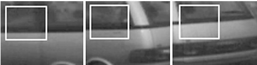
Fig. 4.7 Three images taken at times t , t + 1 , and t + 2 . For the inner rectangles , we may conclude an upward translation with a minor rotation, but the three images clearly indicate a motion of this car to the left
