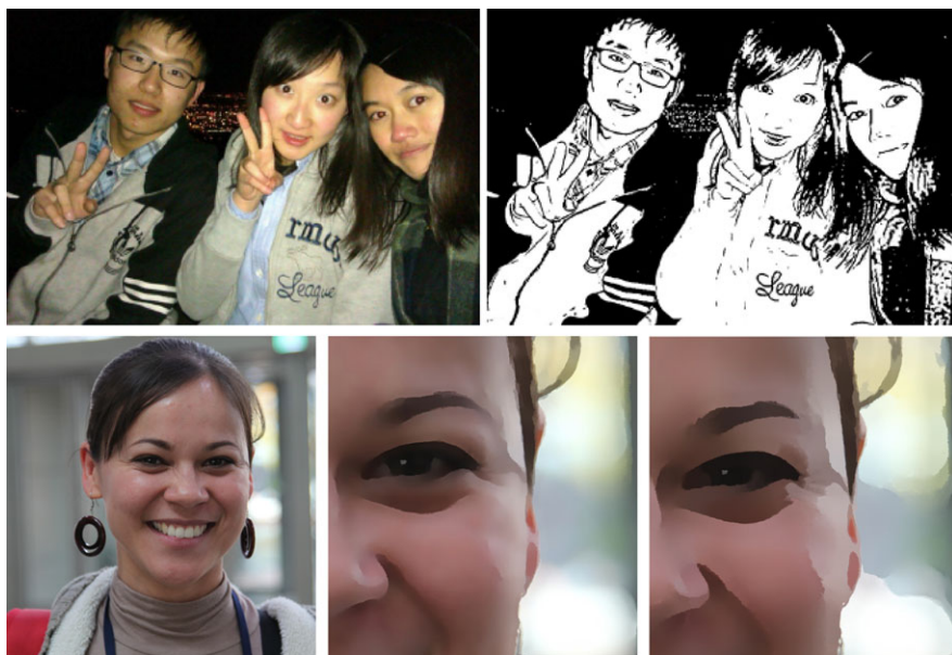
Fig. 5.2 Top: The image AnnieYukiTim ( left ) mapped into a (nearly binary) image defined by Winnemöller stylization. Connected dark or bright regions define segments. Bottom: Segmentation of the image Rocio ( left ) by mean-shift for radii r = 12 ( middle ) and r = 24 ( right ), see text for explanations, showing a window only
