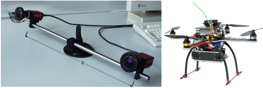
Fig. 6.10 Left: A stereo camera rig on a suction pad with indicated base distance b . Right: A forward-looking stereo camera system integrated into a quadcopter
