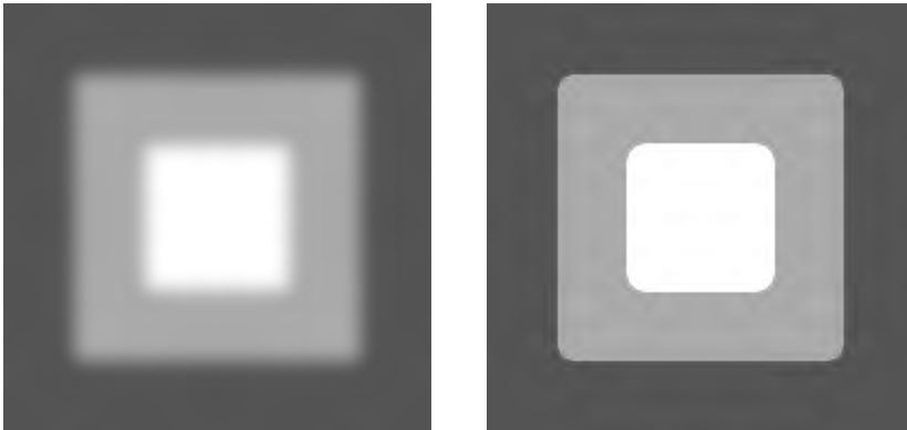
Figure 4.7.1. Blurred image (left) and the result of thresholding it (right).
