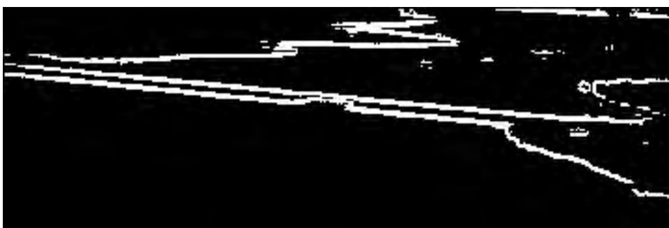
Figure 4.7.5. Result of thresholding Figure 4.7.4 at level specified by maximizing between-class variance.
