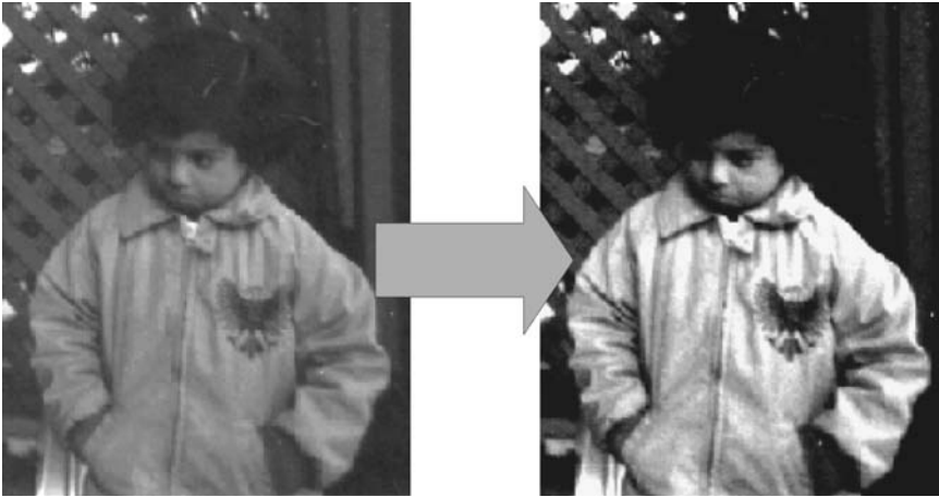
Figure 3.15 Contrast stretch applied to sample image
