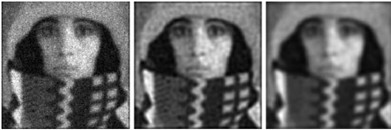
Figure 6.5 Example of constrained deconvolution. Left: original image; centre: restored by minimizing Laplacian of image subject to least-squares noise constraint; right: similar to centre, except Lagrange multiplier fixed at 10 times the previous value
