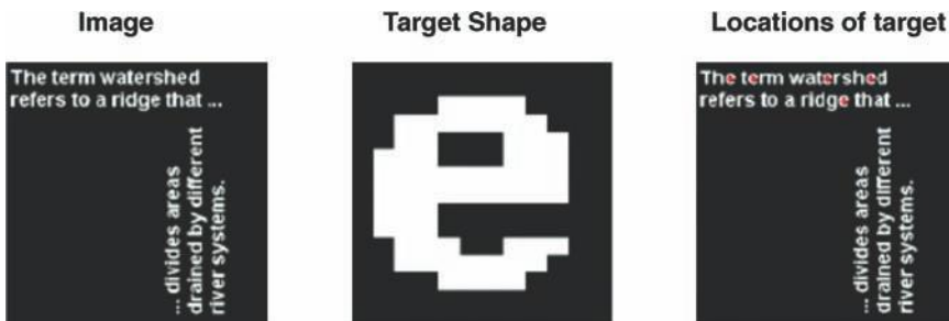
Figure 8.18 Application of the hit-or-miss transformation to detect a target shape in a string of text. Note that the target includes the background and hit-or-miss is strictly sensitive to both the scale and the orientation of the target shape
