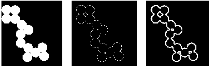
Figure 8.11 Boundary extraction. Left: original.; centre: single-pixel boundary; right: thick boundary extracted through use of larger structuring element
