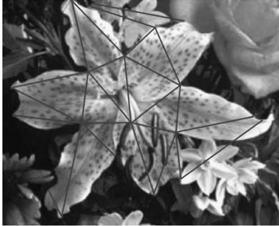
Figure 7.13 Delaunay triangulation divides the image piecewise into contiguous triangular regions. This is a common first stage in piecewise warping
