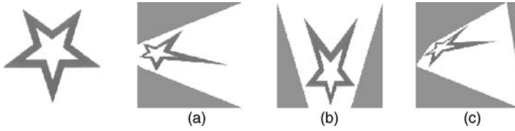
Figure 7.6 Examples of projective transformation. The original image on the left is projectively transformed to examples (a), (b) and (c)
