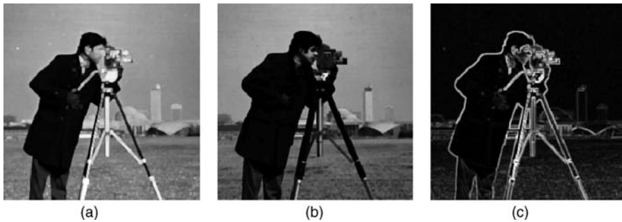
Figure 8.24 Calculating the morphological gradient: (a) grey-scale dilation with flat 3 \times 3 structuring element; (b) grey-scale erosion with flat 3 \times 3 structuring element; (c) difference of (a) and (b) = morphological gradient
