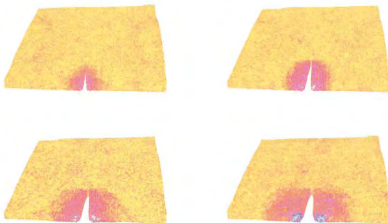
Fig. 5.4. Propagation of a microcrack in silver in two dimensions.
