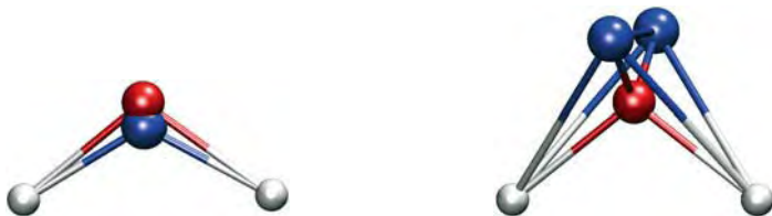
Fig. 7.15. Positions of the centers of mass and charge for four- and five-site models of water.
