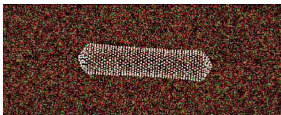
Fig. 5.18. Nanotube-polyethylene composite, relaxed state; the length of the nanotube is 63 Å.
