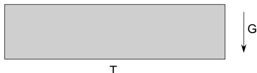
Fig. 3.22. Rayleigh-Bénard convection, configuration with heated lower wall.
